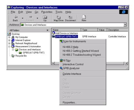
By selecting **Scan for Instruments** in the drop-down menu, you can display all instruments that are powered on and connected to the GPIB board. As shown below, a Tektronix TDS 210 oscilloscope with primary address 1 and a Hewlett-Packard 34970A data acquisition/switch unit with primary address 2 are connected and powered.
