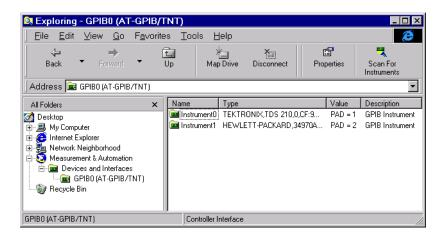
By selecting **NI-488.2 Getting Started Wizard** in the drop-down menu, you can configure the GPIB interface, verify the hardware and software installation, and communicate with the instrument.
