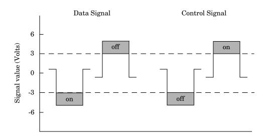
The "on" and "off" states for a data signal and for a control signal are shown below.
